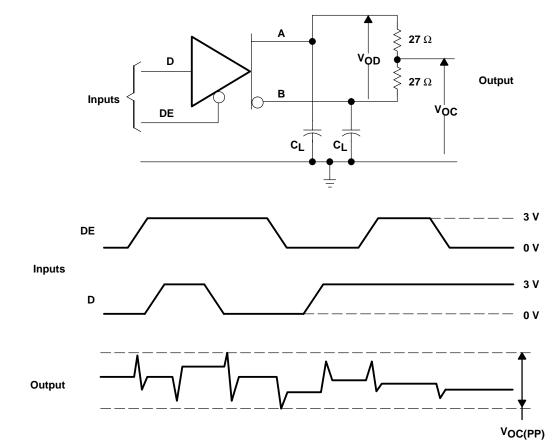
NOTES: A. Resistance values are in ohms and are 1% tolerance. B. C<sub>L</sub> includes probe and jig capacitance ( $\pm$  10%).
