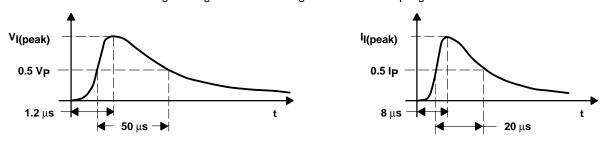
Figure 15. Short-Circuit Current Waveforms
