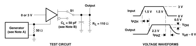
NOTES: A. The input pulse is supplied by a generator having the following characteristics: PRR = 1.25 kHz, 50% duty cycle, t<sub>f</sub>  $\leq$  10 ns, t<sub>f</sub>  $\leq$  10 ns, Z<sub>O</sub> = 50  $\Omega$ .
