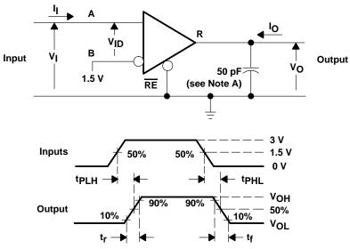
NOTE A: This value includes probe and jig capacitance ( $\pm$  10%).
