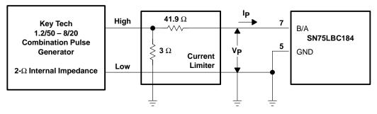
Figure 16. Overvoltage-Stress Test Circuit
